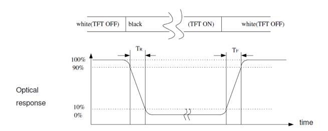
Note (4) Definition of optical measurement setup
